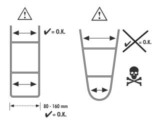
Top-Lock adapter must only be used on carriers with rectanglular base, e.g. left and right rails must be parallel to each other
